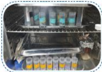
3 Oven drying Measuring bulk density after the oven drying (65°C, 72h)
