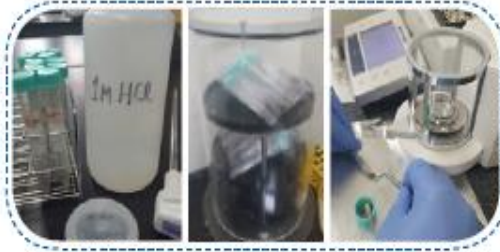
5-2 Freeze-drying Measuring total organic carbon(TOC) content after 1M-HCl treatment and freeze-drying for about 12-24 h
