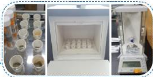
5-1 High temperature drying Measuring organic matter(OM) after drying at 550 °C, 4h
